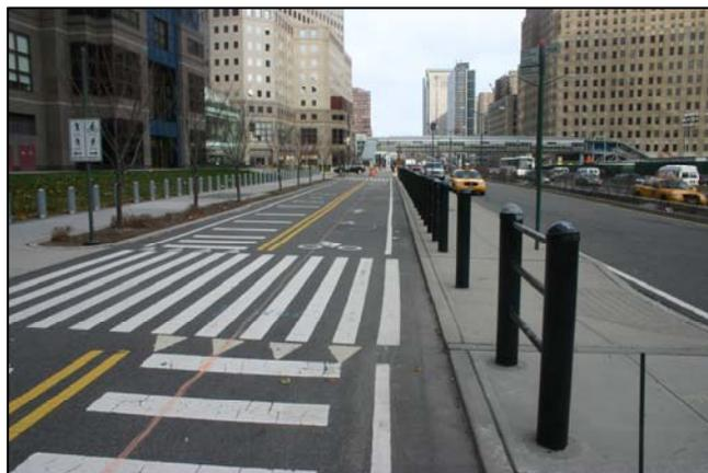
*At the Intrepid Museum, attractive steel bollards protect the plaza from turning tourist coaches and wayward vehicles, while a flexible bollard alerts users to the path entrance (photo, above left). In Lower Manhattan, the Greenway features permanent steel bollards on both sides to protect path users and secure office buildings (photo, below left).*
